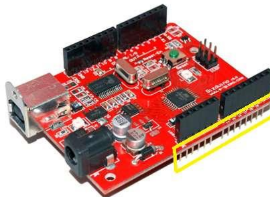
Fig. 2 The Gizduino MCU ATmega324 (Implying the Male Connectors)
